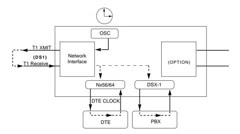
Figure 5-5. Internal Clock Source
